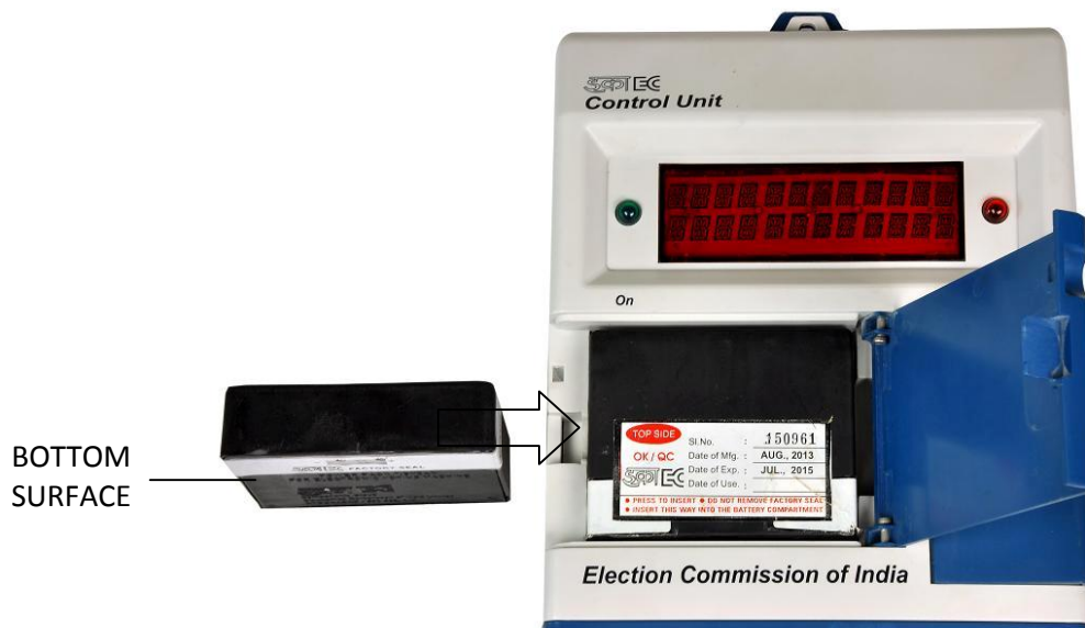
Fig.21 Installing the Power Pack
