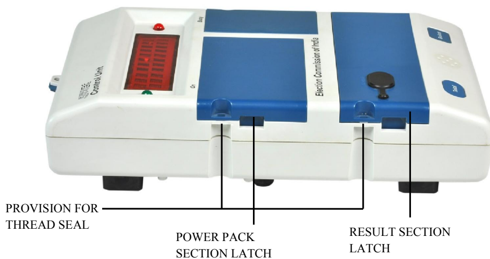
Fig.8 Side View of Control Unit
